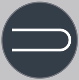
10-12mm diameter steel bar minimum 400mm long
